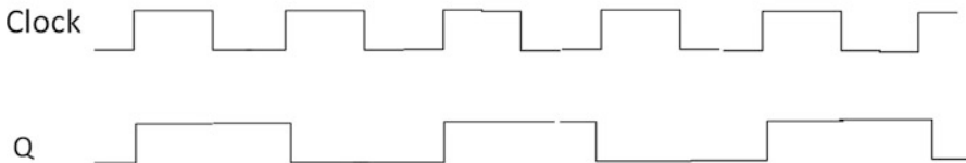
Fig. 5.15 Frequency divider using J-K flip-flop
